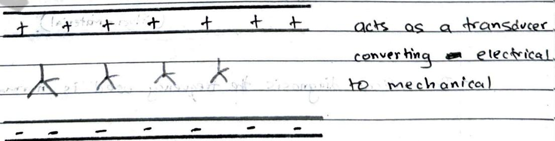
→ an electric field setup in the crystal as the ions are not rigidly held together, they will be displaced due to the force produced by electric field, as opposite ions will attract.
