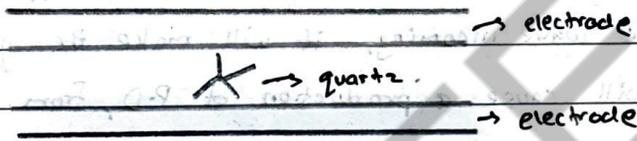
→ when crystals are compressed, the charges are not balanced (positive and negative ions centers do not coincide). PD is created.
